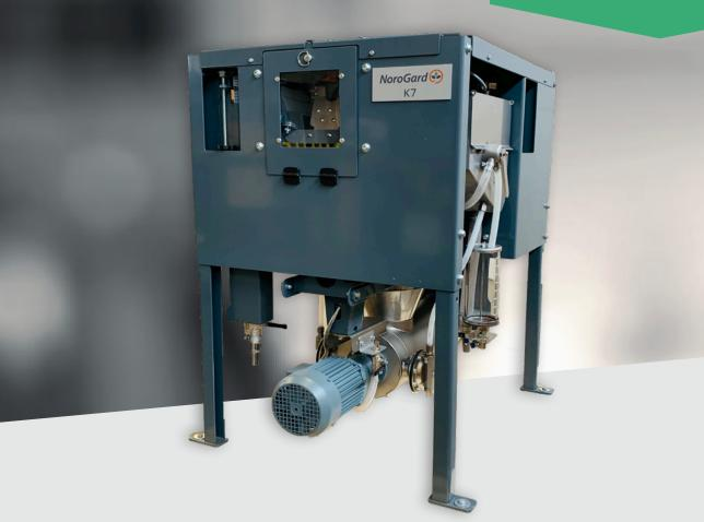
The K7 Continuous Seed Treater is suitable for small and mid sized plants with its variable capacity of up to 7 tons of seed per hour and dosing rates from 100 ml to 2.4 litres per 100 kg seed.
