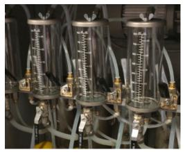
Calibration of the dosage system is easily operated and controlled in a closed system.
